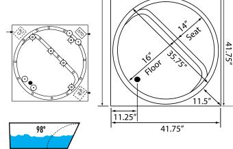
Some standard & most alternate pump locations may stickout past perimeter of the bath 1"-3". NOTE: Graphics may not be to scale. Specifications and features are subject to change without notice and are ± .25". All final measurements should be taken from tub on site. Access 18"x 18" or larger is required for each pump. Consult your contractor for installation requirements.
