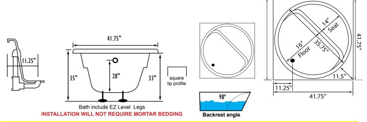
Some standard & most alternate pump locations may stickout past perimeter of the bath 1"-3". NOTE: Graphics may not be to scale. Specifications and features are subject to change without notice and are ± .25". All final measurements should be taken from tub on site. Access 18"x 18" or larger is required for each pump. Consult your contractor for installation requirements.
