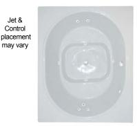
REQUIREMENTS Pump Locations: Select 1 Electrical: one 115v 20AMP GFCI Circuits Tub should not be supported by the lip in any way. Level tub & screw or glue EZ Level adjustable legs to sub floor. **CUT OUT DIMENSIONS: OVALS:** A template will be provided RECTANGLES: Subtract 1" to 1.5" from length & width for hole cut out size
