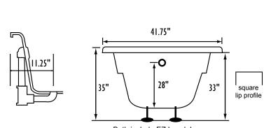
Bath include EZ Level Legs **INSTALLATION WILL NOT REQUIRE MORTAR BEDDING**
