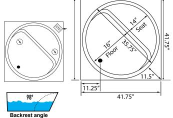
Some standard & most alternate pump locations may stickout past perimeter of the bath 1"-3". NOTE: Graphics may not be to scale. Specifications and features are subject to change without notice and are ± .25". All final measurements should be taken from tub on site. Access 18"x 18" or larger is required for each pump. Consult your contractor for installation requirements.
