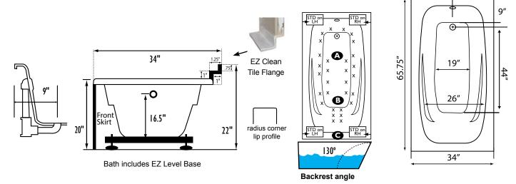
Some standard & most alternate pump locations may stickout past perimeter of the bath 1"-3". NOTE: Graphics may not be to scale. Specifications and features are subject to change without notice and are ± .25". All final measurements should be taken from tub on site. Access 18"x 18" or larger is required for each pump. Consult your contractor for installation requirements.
