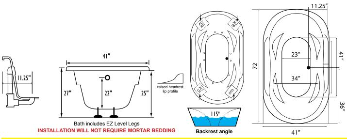
Some standard & most alternate pump locations may stickout past perimeter of the bath 1"-3". NOTE: Graphics may not be to scale. Specifications and features are subject to change without notice and are ± .25". All final measurements should be taken from tub on site. Access 18"x 18" or larger is required for each pump. Consult your contractor for installation requirements.
