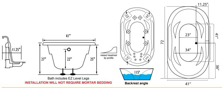
Some standard & most alternate pump locations may stickout past perimeter of the bath 1"-3". NOTE: Graphics may not be to scale. Specifications and features are subject to change without notice and are ± .25". All final measurements should be taken from tub on site.
