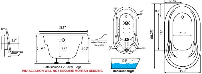
Some standard & most alternate pump locations may stickout past perimeter of the bath 1"-3". NOTE: Graphics may not be to scale. Specifications and features are subject to change without notice and are ± .25". All final measurements should be taken from tub on site. Access 18"x 18" or larger is required for each pump. Consult your contractor for installation requirements.
