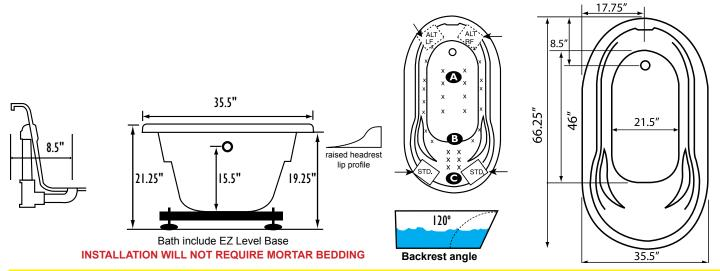
Some standard & most alternate pump locations may stickout past perimeter of the bath 1"-3". NOTE: Graphics may not be to scale.
