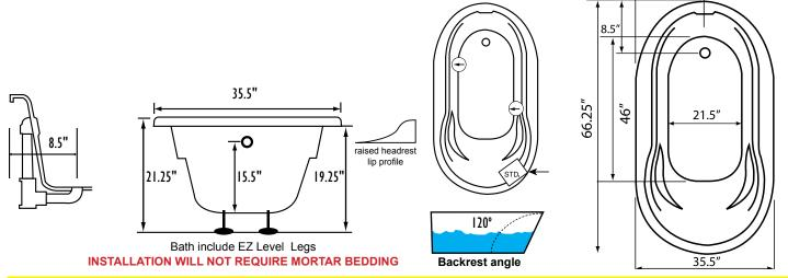
Some standard & most alternate pump locations may stickout past perimeter of the bath 1"-3". NOTE: Graphics may not be to scale. Specifications and features are subject to change without notice and are ± .25". All final measurements should be taken from tub on site.
