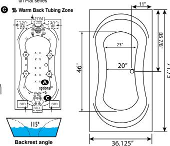
Some standard & most alternate pump locations may stickout past perimeter of the bath 1"-3". NOTE: Graphics may not be to scale. Specifications and features are subject to change without notice and are ± .25". All final measurements should be taken from tub on site. Access 18"x 18" or larger is required for each pump. Consult your contractor for installation requirements.
