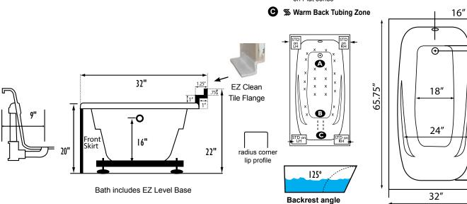
Some standard & most alternate pump locations may stickout past perimeter of the bath 1"-3". NOTE: Graphics may not be to scale.
