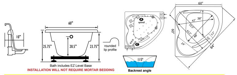
Some standard & most alternate pump locations may stickout past perimeter of the bath 1"-3". NOTE: Graphics may not be to scale. Specifications and features are subject to change without notice and are ± .25". All final measurements should be taken from tub on site.
