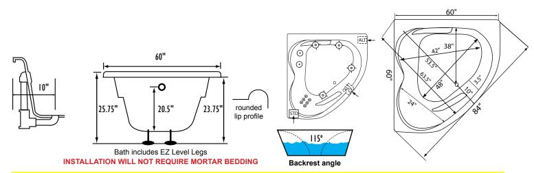
Some standard & most alternate pump locations may stickout past perimeter of the bath 1"-3". NOTE: Graphics may not be to scale. Specifications and features are subject to change without notice and are ± .25". All final measurements should be taken from tub on site.
