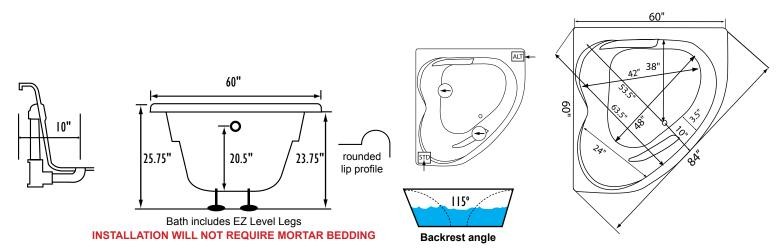
Some standard & most alternate pump locations may stickout past perimeter of the bath 1"-3". NOTE: Graphics may not be to scale. Specifications and features are subject to change without notice and are ± .25". All final measurements should be taken from tub on site. Access 18"x 18" or larger is required for each pump. Consult your contractor for installation requirements.
