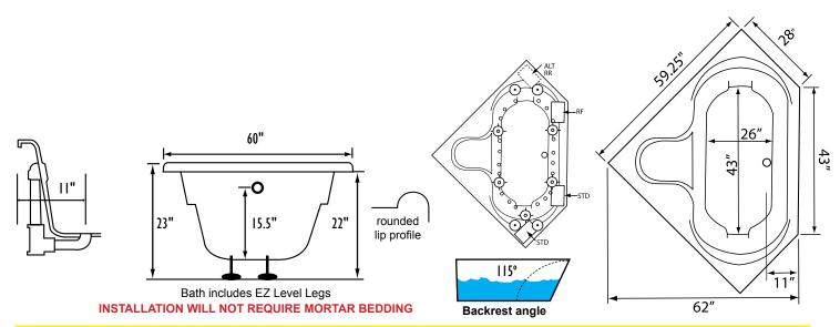
Some standard & most alternate pump locations may stickout past perimeter of the bath 1"-3". NOTE: Graphics may not be to scale.
