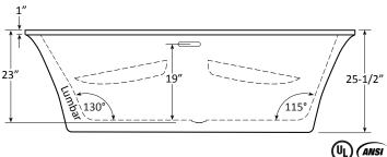
Specifications and features are subject to change without notice and are + .25". All final measurements should be taken from tub on site. HydroMassage Products LLC • 303-341-1845 • Fax: 303-341-1850 • www.hydromassageproducts.com
