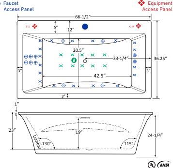
Specifications and features are subject to change without notice and are + .25". All final measurements should be taken from tub on site. HydroMassage Products LLC • 303-341-1845 • Fax: 303-341-1850 • www.hydromassageproducts.com
