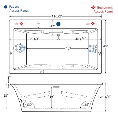
Specifications and features are subject to change without notice and are + .25". All final measurements should be taken from tub on site. HydroMassage Products LLC • 303-341-1845 • Fax: 303-341-1850 • www.hydromassageproducts.com
