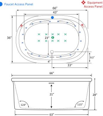
Specifications and features are subject to change without notice and are + .25". All final measurements should be taken from tub on site. HydroMassage Products LLC • 303-341-1845 • Fax: 303-341-1850 • www.hydromassageproducts.com
