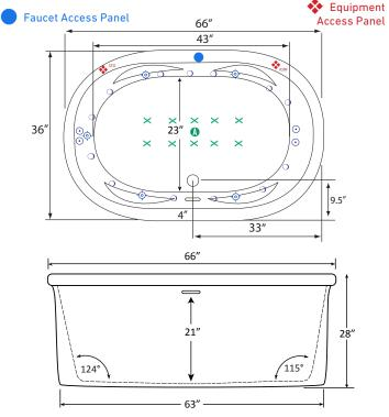
Specifications and features are subject to change without notice and are + .25". All final measurements should be taken from tub on site. HydroMassage Products LLC • 303-341-1845 • Fax: 303-341-1850 • www.hydromassageproducts.com
