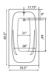
Bath include EZ Level Legs **INSTALLATION WILL NOT REQUIRE MORTAR BEDDING**
