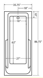
Some standard & most alternate pump locations may stickout past perimeter of the bath 1"-3". NOTE: Graphics may not be to scale. Specifications and features are subject to change without notice and are ± .25". All final measurements should be taken from tub on site.
