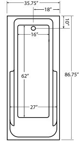
Some standard & most alternate pump locations may stickout past perimeter of the bath 1"-3". NOTE: Graphics may not be to scale. Specifications and features are subject to change without notice and are ± .25". All final measurements should be taken from tub on site. Access 18"x 18" or larger is required for each pump. Consult your contractor for installation requirements.
