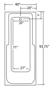
Some standard & most alternate pump locations may stickout past perimeter of the bath 1"-3". NOTE: Graphics may not be to scale. Specifications and features are subject to change without notice and are ± .25". All final measurements should be taken from tub on site.
