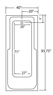
Some standard & most alternate pump locations may stickout past perimeter of the bath 1"-3". NOTE: Graphics may not be to scale. Specifications and features are subject to change without notice and are ± .25". All final measurements should be taken from tub on site. Access 18"x 18" or larger is required for each pump. Consult your contractor for installation requirements.
