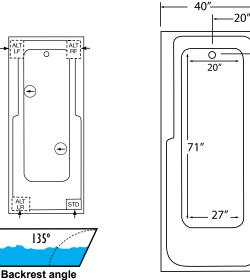
Some standard & most alternate pump locations may stickout past perimeter of the bath 1"-3". NOTE: Graphics may not be to scale. Specifications and features are subject to change without notice and are ± .25". All final measurements should be taken from tub on site. Access 18"x 18" or larger is required for each pump. Consult your contractor for installation requirements.
