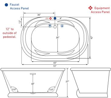
Decorative Pedestal is not on back side in order to accommodate equipment access. This side should be placed against wall.
