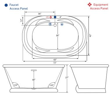
Decorative Pedestal is not on back side in order to accommodate equipment access. This side should be placed against wall.
