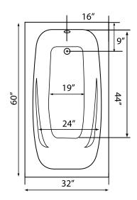
Bath include EZ Level Base **INSTALLATION WILL NOT REQUIRE MORTAR BEDDING**
