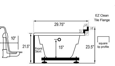
Bath includes EZ Level Base INSTALLATION WILL NOT REQUIRE MORTAR BEDDING
