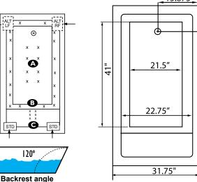
Some standard & most alternate pump locations may stickout past perimeter of the bath 1"-3". NOTE: Graphics may not be to scale. Specifications and features are subject to change without notice and are ± .25". All final measurements should be taken from tub on site. Access 18"x 18" or larger is required for each pump. Consult your contractor for installation requirements.
