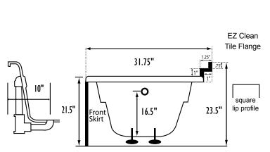
Bath includes EZ Level Legs **INSTALLATION WILL NOT REQUIRE MORTAR BEDDING**
