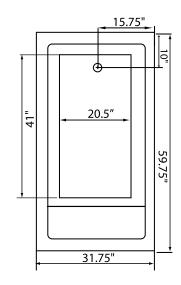
Some standard & most alternate pump locations may stickout past perimeter of the bath 1"-3". NOTE: Graphics may not be to scale. Specifications and features are subject to change without notice and are ± .25". All final measurements should be taken from tub on site. Access 18"x 18" or larger is required for each pump. Consult your contractor for installation requirements.
