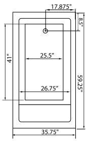
Some standard & most alternate pump locations may stickout past perimeter of the bath 1"-3". NOTE: Graphics may not be to scale. Specifications and features are subject to change without notice and are ± .25". All final measurements should be taken from tub on site.
