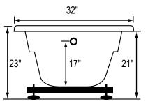
Bath includes EZ Level Base INSTALLATION WILL NOT REQUIRE MORTAR BEDDING
