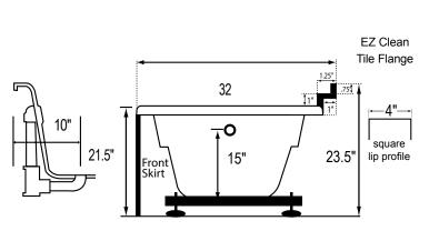
Bath includes EZ Level Base INSTALLATION WILL NOT REQUIRE MORTAR BEDDING
