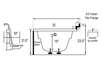
Bath includes EZ Level Legs **INSTALLATION WILL NOT REQUIRE MORTAR BEDDING**
