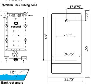
Some standard & most alternate pump locations may stickout past perimeter of the bath 1"-3". NOTE: Graphics may not be to scale. Specifications and features are subject to change without notice and are ± .25". All final measurements should be taken from tub on site.
