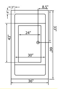
Some standard & most alternate pump locations may stickout past perimeter of the bath 1"-3". NOTE: Graphics may not be to scale. Specifications and features are subject to change without notice and are ± .25". All final measurements should be taken from tub on site.
