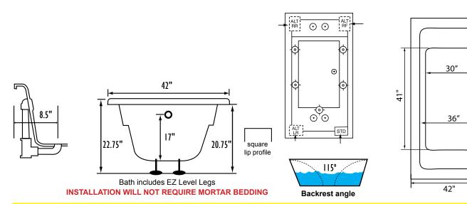
Some standard & most alternate pump locations may stickout past perimeter of the bath 1"-3". NOTE: Graphics may not be to scale. Specifications and features are subject to change without notice and are ± .25". All final measurements should be taken from tub on site. Access 18"x 18" or larger is required for each pump. Consult your contractor for installation requirements.
