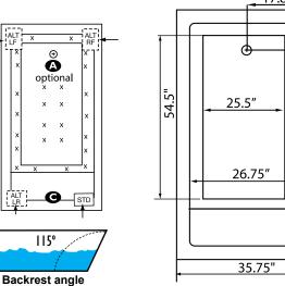
Some standard & most alternate pump locations may stickout past perimeter of the bath 1"-3". NOTE: Graphics may not be to scale. Specifications and features are subject to change without notice and are ± .25". All final measurements should be taken from tub on site.
