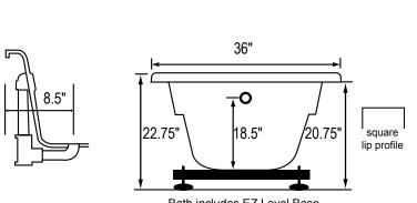
Bath includes EZ Level Base INSTALLATION WILL NOT REQUIRE MORTAR BEDDING
