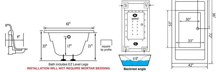
NOTE: Graphics may not be to scale. Specifications and features are subject to change without notice and are ± .25". All final measurements should be taken from tub on site. Access 18"x 18" or larger is required for each pump. Some pump locations and plumbing may extend beyond the perimeter of the bath.
