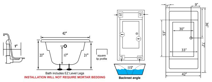
**NOTE:** Graphics may not be to scale. Specifications and features are subject to change without notice and are ± .25". All final measurements should be taken from **tub on site.** Access 18"x 18" or larger is required for each pump. Some pump locations and plumbing may extend beyond the perimeter of the bath.
