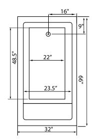
Some standard & most alternate pump locations may stickout past perimeter of the bath 1"-3". NOTE: Graphics may not be to scale. Specifications and features are subject to change without notice and are ± .25". All final measurements should be taken from tub on site. Access 18"x 18" or larger is required for each pump. Consult your contractor for installation requirements.
