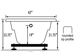
Bath include EZ Level Base INSTALLATION WILL NOT REQUIRE MORTAR BEDDING
