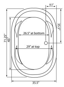
Bath includes EZ Level Legs **INSTALLATION WILL NOT REQUIRE MORTAR BEDDING**
