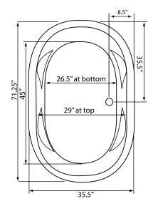
Some standard & most alternate pump locations may stickout past perimeter of the bath 1"-3". NOTE: Graphics may not be to scale. Specifications and features are subject to change without notice and are ± .25". All final measurements should be taken from tub on site. Access 18"x 18" or larger is required for each pump. Consult your contractor for installation requirements.
